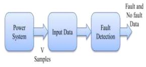
Fig: 3 Major blocks constituting the fault detector
