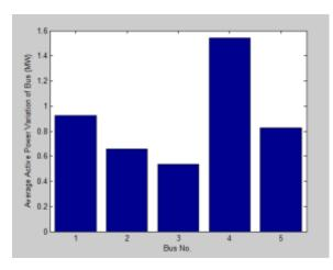
Fig: 5 Waveform of Classified Active Power 'P' for fault between phase 'a' and Ground at BusesBus 1: 0.9229Bus 2: 0.6560Bus 3: 0.5361Bus 4: 1.5431Bus 5: 0.8278
