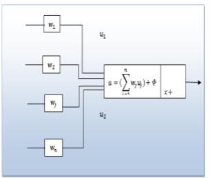
Fig: 1 Artificial Neuron Network Model
